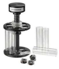
Six tubes opened at the upper end and closed by a screen at the lower
